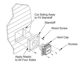
Figure 11 - Installing Siding Standoff (Combustible Exterior)
